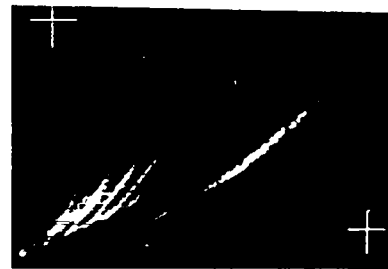
Fig. VII-5. Image of ion tracks obtained by (a) conventional contact photography and (b) dark-field illumination.
